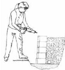
A perforated drainage pipe must be placed at the base of the wall and must be sloped toward a catch basin or drainage area.
