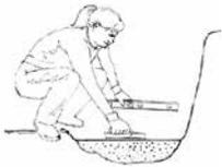
5. Lay your first course using a string line to help with alignment. Place each unit edge-to-edge, lining up the back of the units with the string. For smooth curves use flexible 1" PVC pipe as your guide.
