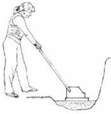
3. Fill the trench with 4 inches of well-graded gravel material, (1/2" minus or 3/4" minus road mulch) compacting firmly in 2-inch layers to ensure proper compaction. Note: Hand tamping tools may be used, but vibrating compaction equipment is recommended.
